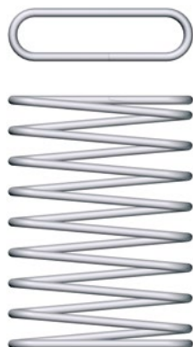
9. Rectangularly wound compression spring (magazine spring)
