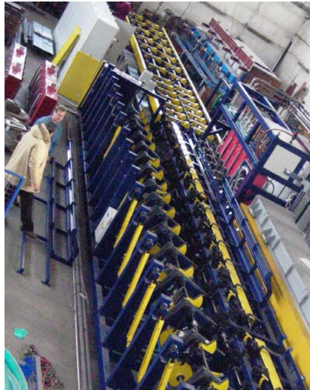
Part of the induction heating line under assembling.
