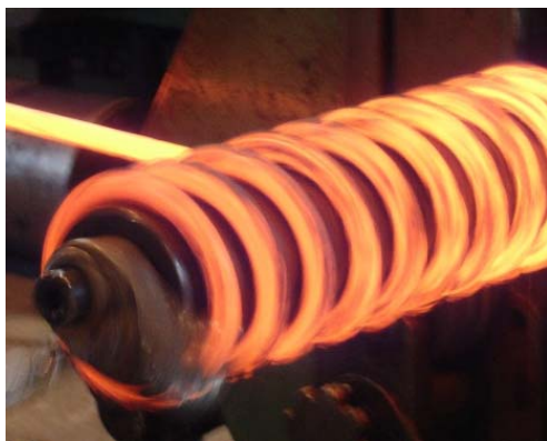
Hot bar under coiling before quenching.
